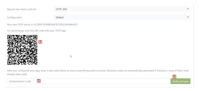
4: After the QR code has been generated, it must be scanned in the TOTP app (MS or Google Authenticator). The app will now generate a new password every 30 seconds.
